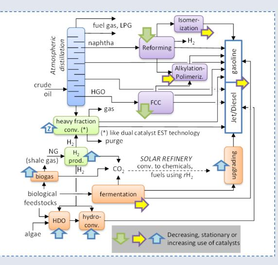
Fig. 1 Schematic diagram of possible future integrated scheme of energy vectors production (refinery). Solar refinery deals with the conversion of  $CD_2$  to chemicals using renewable  $H_2$  (see figure 2). Source. Catal. Science & Techn., 2016, 6, 2485.
