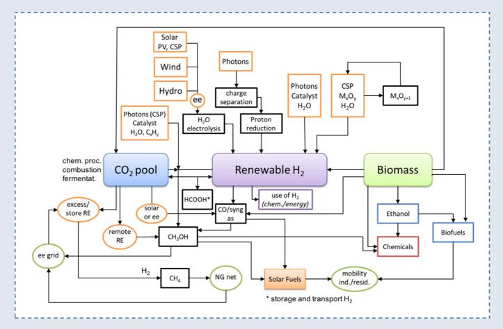
Fig. 2 The solar (bio)refinery concept for chemical energy storage science and technologies. Modified from the original presented by Schlögl<sup>1</sup>
